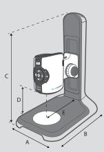
Ergo stand dimensions: **A** = 11" (280mm) **B** = 16.5" (420mm) **C** = 20.3" (515mm) **D** = 7.6" (192mm) max. **E** = 7.9" (200mm)
