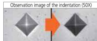
Stray light reduction around the indentation
