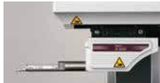
178-071 (S-3000) Standard Detector Holder
