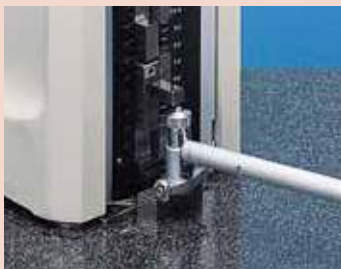
Bore gage zero-setting
