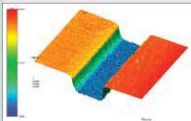
3-dimensional topographical result, data of micro-circuit
