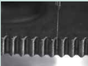
Measuring form of micro gear teeth
