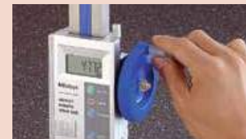
Large, smooth slider-feed wheel
