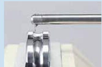
Inner/outer ring contour of a bearing
