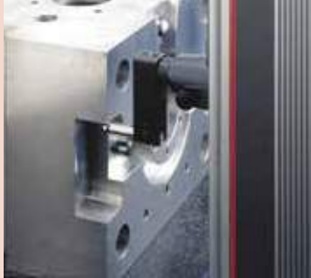
12AAF668 ø10 ball probe, L=82
